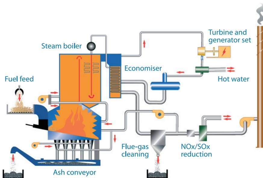
Example of a KMW Energi cogeneration plant for the production of electricity and district heating, with corresponding environmental systems.
