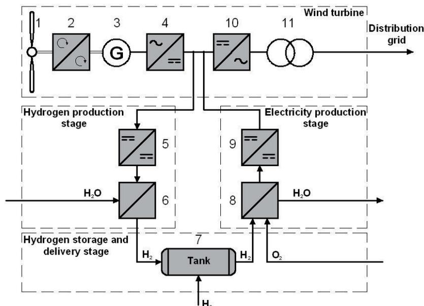
**Fig. 3.** Block diagram of the proposed hydrogen buffer: 1 – Blades; 2 - Gearbox; 3 - Generator; 4 – Rectifier; 5 - Interface DC/DC converter, 6 – Electrolyser; 7 - Storage tank; 8 - Fuel cell; 9 - Interface DC/DC converter; 10 – Inverter; 11 - Transformer.
