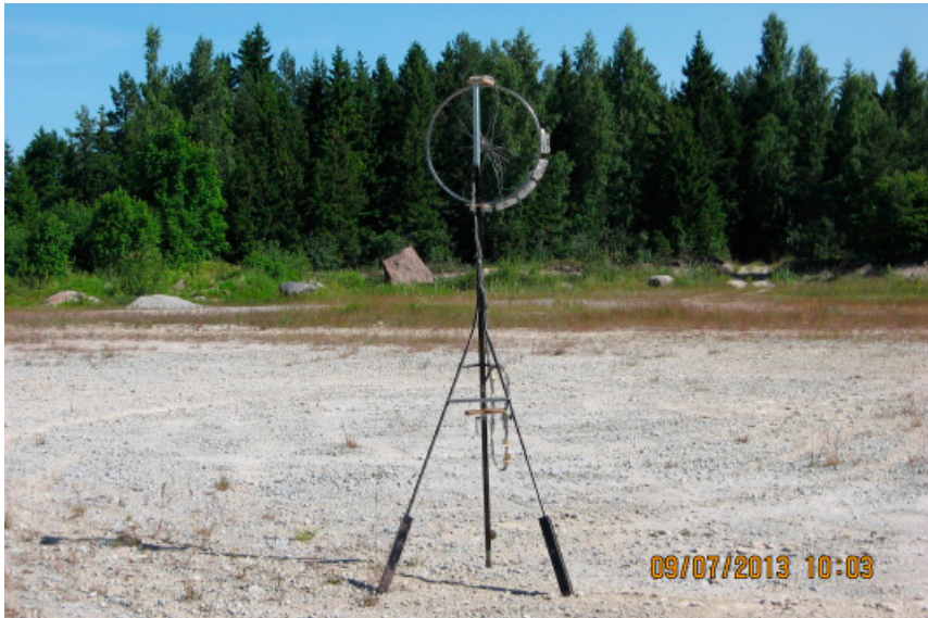
Joonis 2. Eksperimentaalne mõõtestend, kohandatuna kalletele 90^{\circ} < \beta < 180^{\circ} Figure 2. Experimental measurements stand, justified for tilt angles 90^{\circ} < \beta < 180^{\circ}
