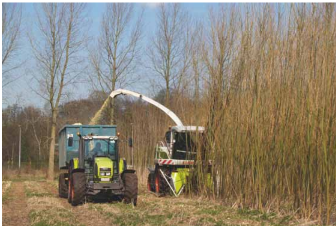
Joonis 3. Võsakoristuskombain CLAAS Jaguar (CLAAS Europe 2009) Figure 3. Wood-chopper CLAAS Jaguar (CLAAS Europe 2009)
