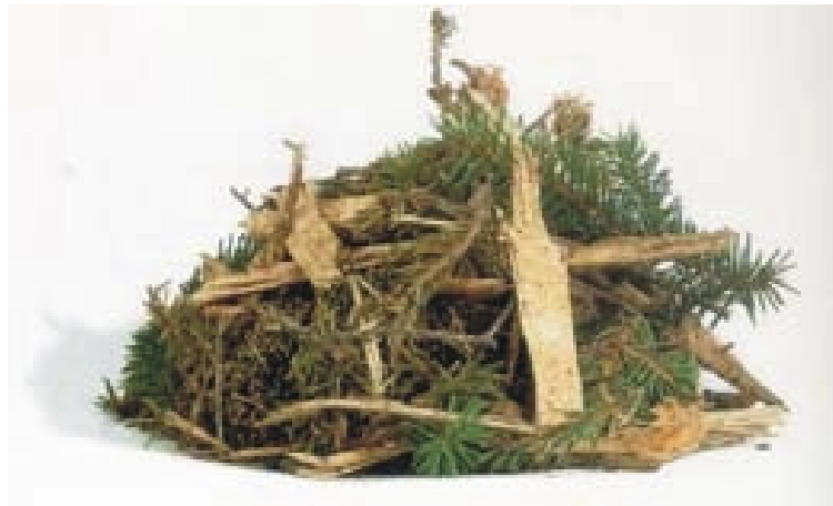
Joonis 2. Metsajäätmed; W^t = 45\text{--}60\% , Q_a^t = 6\text{--}9 \text{ MJ/kg} , A^k = 1\text{--}3\% Figure 2. Forest residue; W^t = 45\text{--}60\% , Q_a^t = 6\text{--}9 \text{ MJ/kg} , A^k = 1\text{--}3\%
