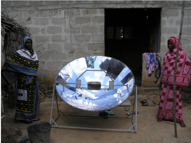
Picture 2: Typical parabolic concentrating solar cooker in Zanzibar (by Pia Otte, 2008)
