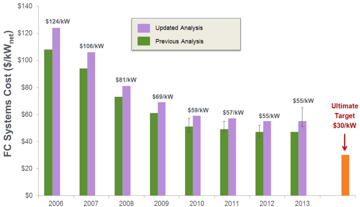
Figure 2. Modeled cost of an 80-kW net PEM fuel cell system based on projection to high-volume manufacturing (500,000 units/year). Reported values from prior year cost estimates were adjusted to account for the higher platinum price, the realigned compressor and expander efficiencies, and the Q/ΔT requirement introduced in 2013.
