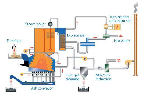
Example of a KMW Energi cogeneration plant for the production of electricity and district heating, with corresponding environmental systems. Source: KMW Energi, Sweden
