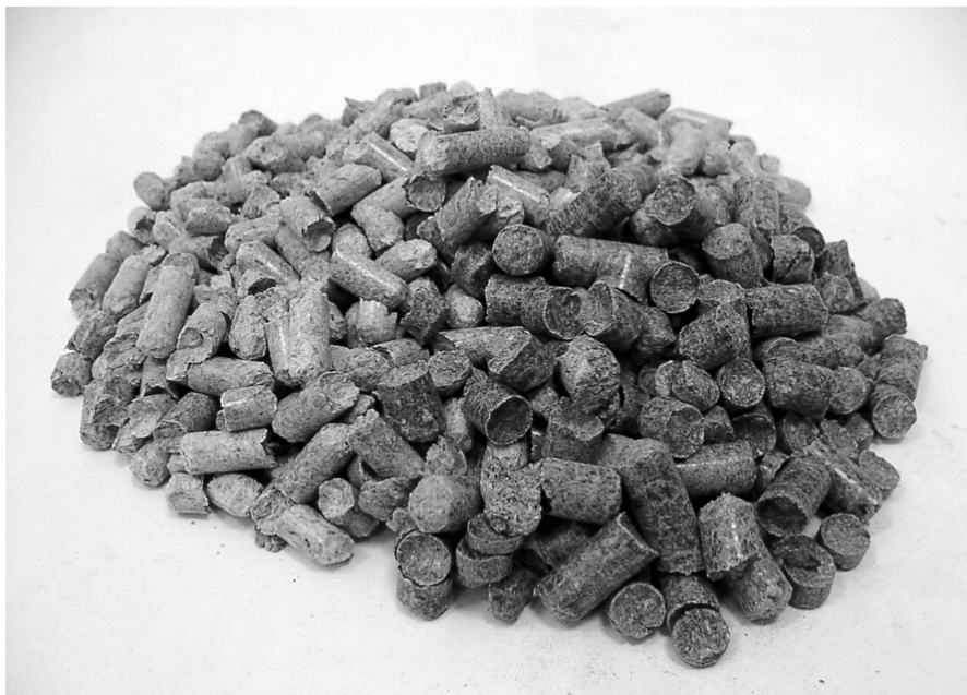
Joonis 4. Puitgraanulid (pelletid); W^t = <10\% , Q_a^t = 16,5-18 \text{ MJ/kg} , A^k = <1,5\% , S^k < 0,05\% , N^k = <0,3\% , Cl^k < 0,03\% Figure 4. Wood pellets; W^t = <10\% , Q_a^t = 16,5-18 \text{ MJ/kg} , A^k = <1,5\% , S^k < 0,05\% , N^k = <0,3\% , Cl^k < 0,03\%
