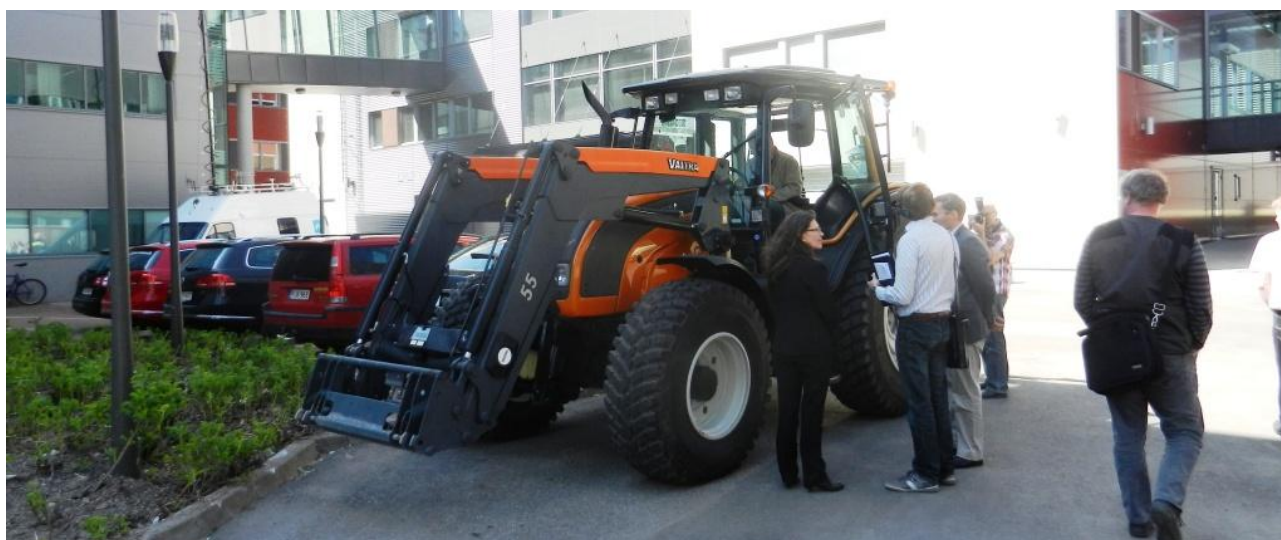
Figure 2.11. Valtra dualfuel-diesel biogas (CBG) agricultural tractor at 3rd Finnish Traffic Biogas Conference and Exhibition in Joensuu, 28 May 2012. It can also use biodiesel (B100).
